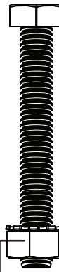
H-7 M6 x 45mm Hex Bolt and M6 Nut with Tooth Washer
